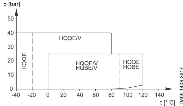
**Fig. 8** Operating range of standard shaft seals for  $\varnothing 28$  shaft ends (75-110 kW)
