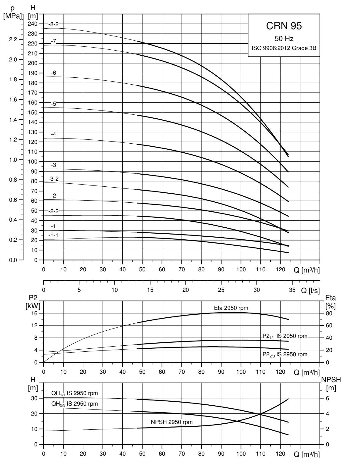
The maximum pump efficiency (ETA) is based on a three-stage pump.
