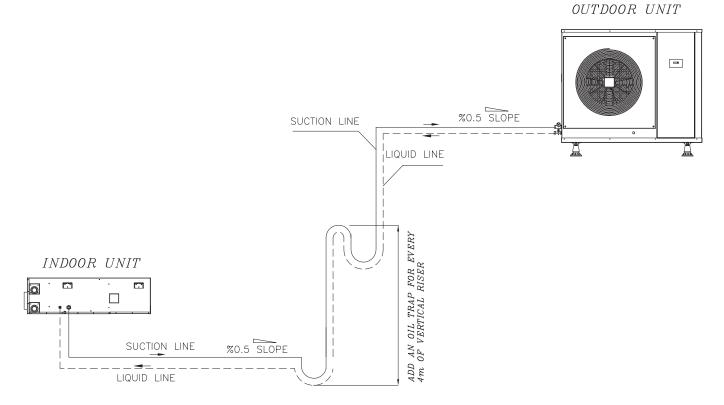
• If the indoor unit lies above the outdoor unit, the suction line must have a loop at the indoor unit's outlet to prevent refrigerant from draining into the compressor during off-cycles.
